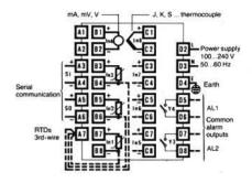
Supply: D2 and D3; D4 (earth) Inputs (note 1): B1...B8 for inputs 1. C1...C8 for inputs 5...8 A7: Common RTDs 3rd-wire. For a 2-wire connection, jump the negative terminal of the input to this terminal Serial communication: A3 and A4 reception A5 and A6 transmission Common alarm Y4: D5 and D6 (AL1) Common alarm Y3: D7 and D8 (AL2)
