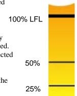
However, a process oven or oxidizer is allowed to operate with only a 2:1 safety margin (up to 50% of the LFL), when continuous flammability analyzers are used. The requirements stipulate real-time, fast-response, *continuous* analyzers connected in such a manner as to trigger corrective action at predetermined alarm points.
