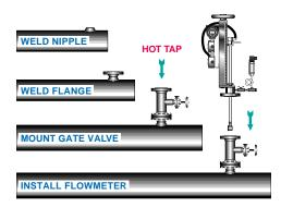
Insertion flowmeters can be installed quickly and easily, reducing costs. The "hot tap capability" allows EMCO insertion flowmeters to be installed and serviced without process shutdown; a feature that not only saves on labor costs, but also avoids disruption of a critical process.
