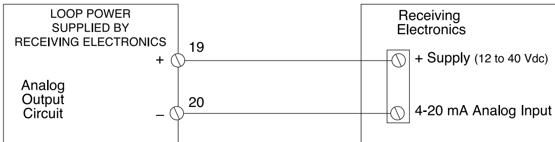
Figure 6. 4-20 mA Current Source Analog Output
