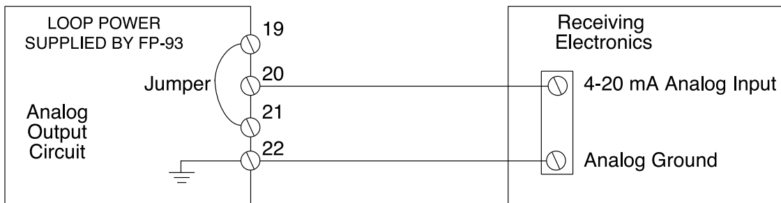
Figure 5. 4-20 mA Isolated Analog Output
