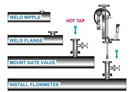
Insertion flowmeters can be installed quickly and easily, reducing costs. The "hot tap capability" allows EMCO insertion flowmeters to be installed and serviced without process shutdown; a feature that not only saves on labor costs, but also avoids disruption of a critical process.
