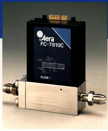
The FC-7800 series MFC's have demonstrated excellent performance in the most demanding applications for a number of years, and these MFC's still surpass the performance of the most advanced models of competitive MFC manufacturers. The FC-7800 series is designed for use in processes where reactive gases may degrade elastomer seals or where superior leak integrity is required. An optional electropolishing and ultracleaning treatment for the base, bypass nut and fittings is available.
