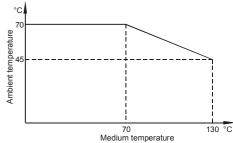
suspended solids or material that could stick between the float and the guide rod. If used at temperatures in exess of 70 °C the maximum ambient temperature allowed will be in accordance with the derating diagram.
