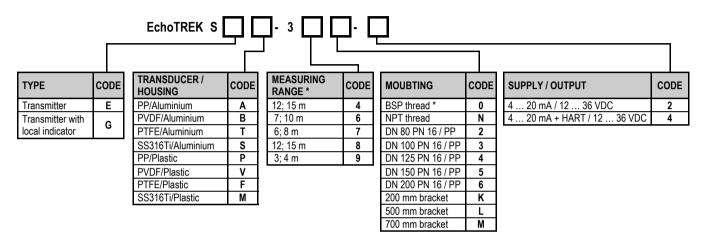
\* Measuring range depends on the material of the transducer
