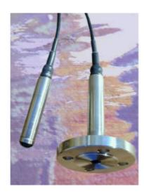
The PSM Series 700 Borehole and Probe Transmitters employ the proven principle of pressure sensitive diaphragm and LVDT. They are specifically designed for applications where access for installation is restricted such as deep wells or buried storage vessels.
